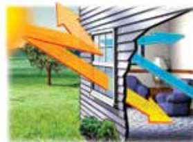
In summer months, Low-E insulating glass helps block unwanted solar heat penetration to conserve air-conditioning use.
