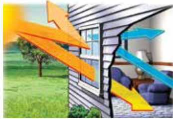
Summer Energy Savings: Low-E helps block unwanted solar heat penetration to help conserve air-conditioning use.
