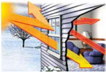
Winter Energy Savings: Low-E insulating glass reduces heat loss by reflecting warmth back into your home.
