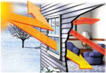
Winter Energy Savings: Low-E insulating glass reduces heat loss by reflecting warmth back into your home.
